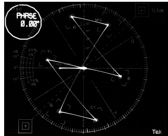
A vectorscope display of color bars.
